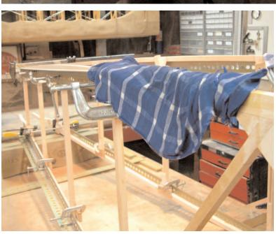
The firewall and all major cross beams, including the massive lamination that forms the front of the cockpit, were made first in a jig, and pre-drilled (top left).
