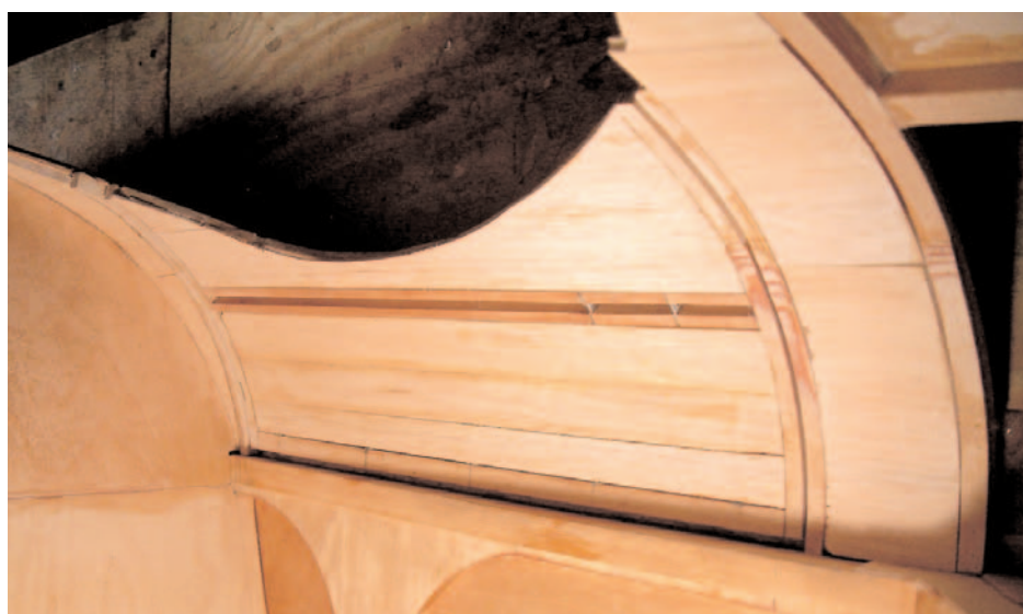
The cockpit door was built in place with balsa filling in preparation for cutting it out. The lower member left room for the hinge, and incorporated T-nuts for the hinge attachment screws.
