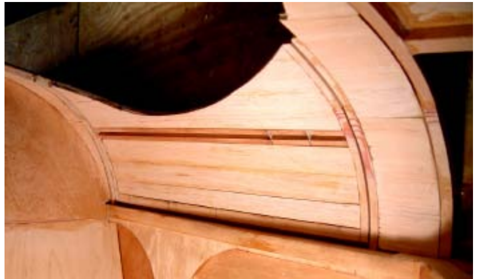
The cockpit door was built in place with balsa filling in preparation for cutting it out. The lower member left room for the hinge, and incorporated T-nuts for the hinge attachment screws.
