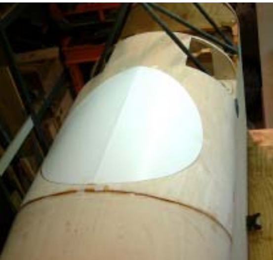
The cockpit opening was marked and cut out.
