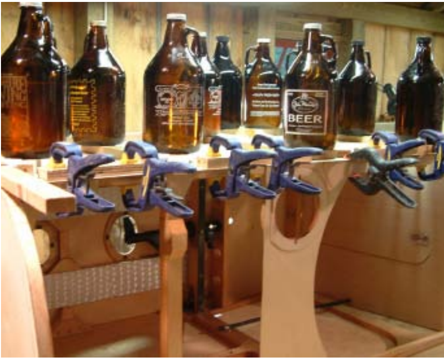
Emergency clamping: Growlers can provide up to 4 lbs each of versatile, localized pressure.
