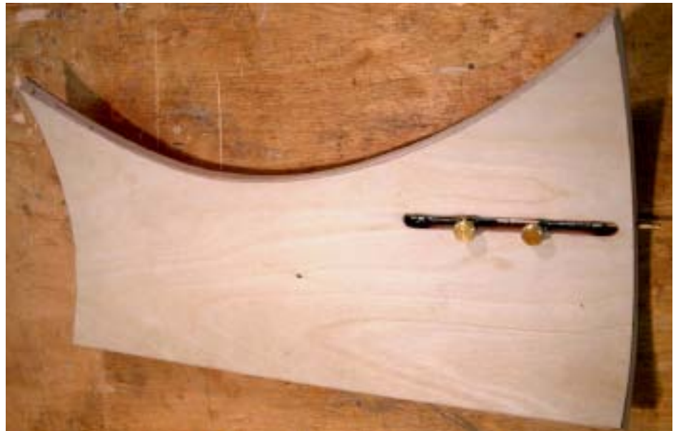
The latch was built in, plywood liner attached. Cutting out was with a hacksaw blade and a sharp knife.
