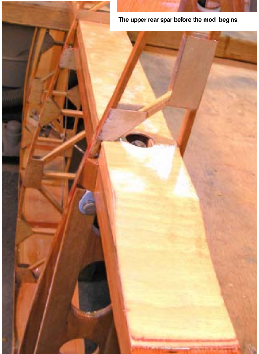
Ribs reconstructed, and good to go to 6.6 g for gentlemanly aerobatics on a Sunday afternoon.
