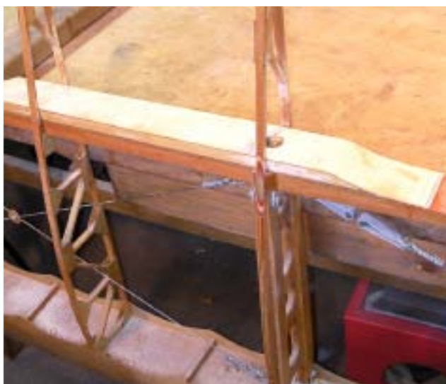
Reinforcing strips are boxed in with 1.5 mm plywood.
