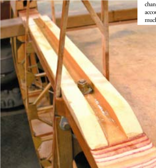
Rib structure is cut away and reinforcing strips glued on.
