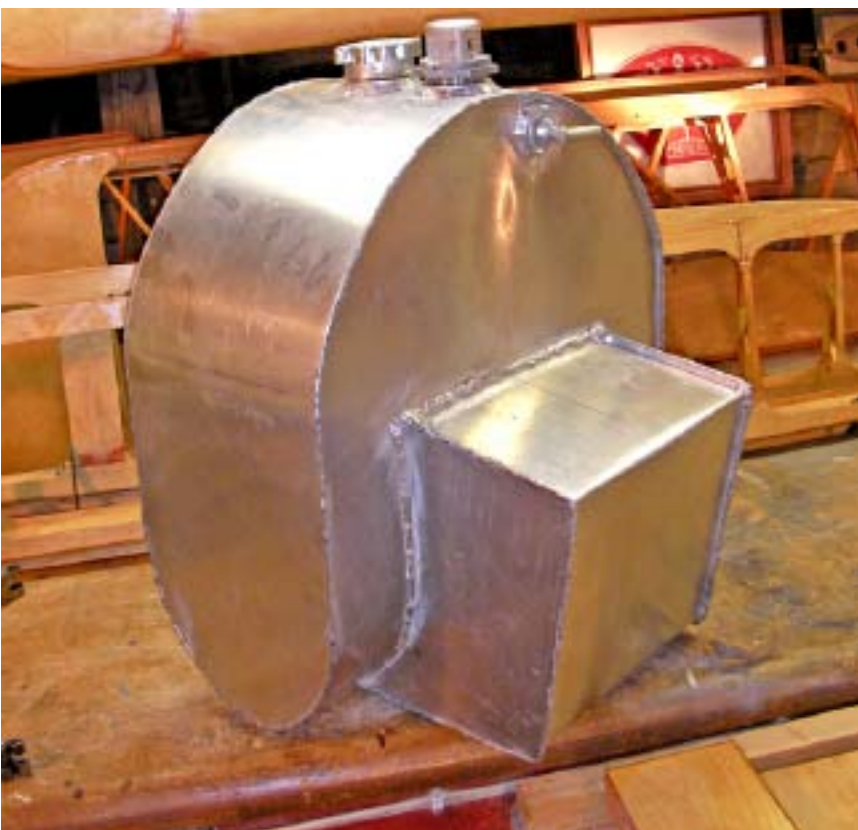
The 14 gallon (U.S.) fuel tank boasts a rotating gauge and a vent for inverted flight.
