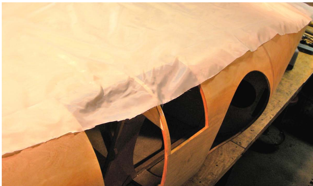
A length of Ceconite fabric is sized and cut to cover the whole side of the fuselage up to the decking in one piece.
