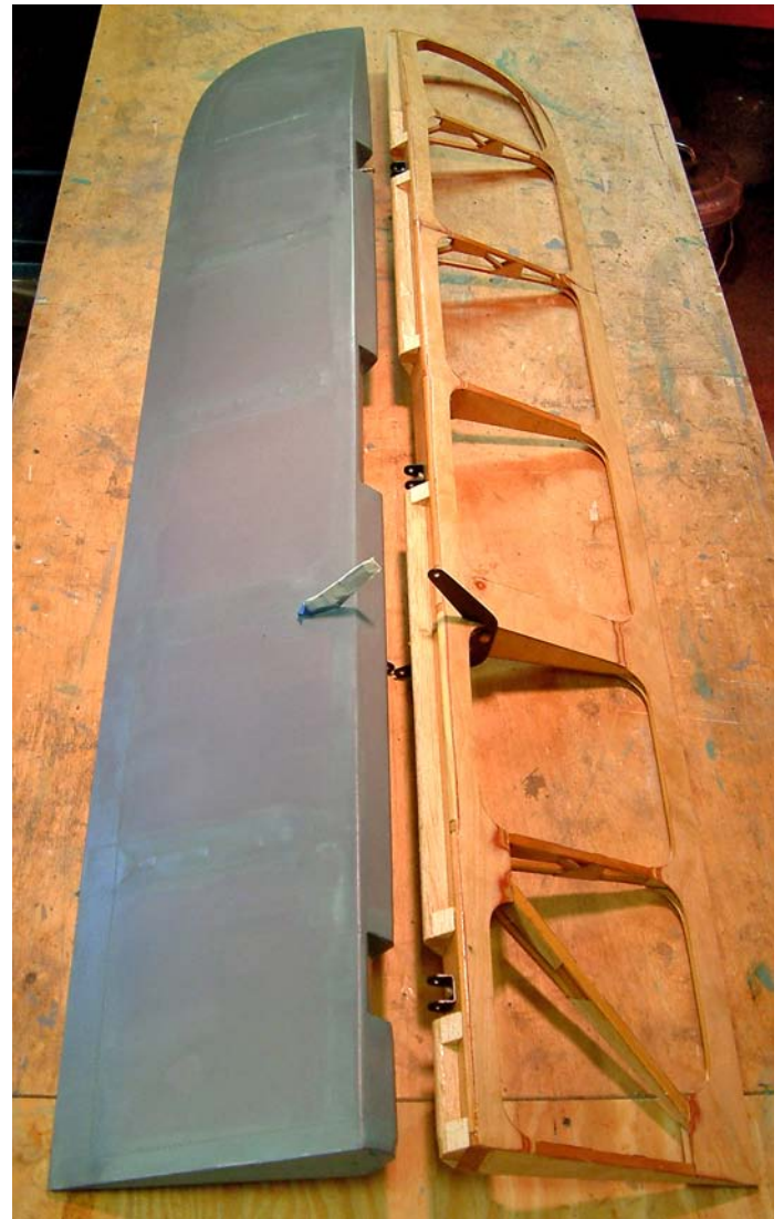
The ailerons acquire a nice rounded leading adge after being covered.
