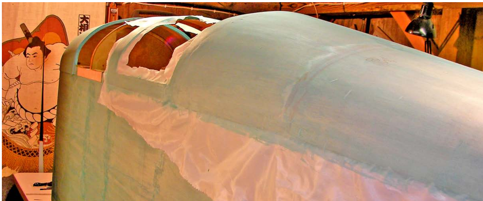
Sides covered, Ceconite is now fitted and glued to the upper decking, with great care being taken with the cosmetics around the cockpit opening as these will show later.
