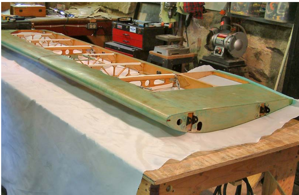
The lower wings were covered in one piece of Ceconite, from trailing edge, over the leading edge, and back.
