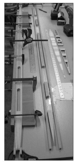
ELEVATOR TRIAL FITTED. ELEVATOR AND TAIL PLANE SPAR GET-TING READY FOR GLUE (DRY RUN HERE). ELEVATOR AND TAIL PLANE SPAR ARE SIMILAR BUT NOT IDENTICAL TO EACH OTHER THE TAIL PLANE RIB AND ELEVATOR RIB COULD BE SEEN TO THE RIGHT.
