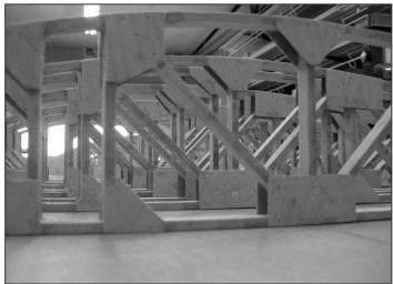
THE UPPER AND LOWER WING RIBS ARE ALMOST COMPLETED. ONLY NEED TO FORM RIB NOSE AND CUT THE END. THE LOWER OUTER RIBS WERE SIMPLIFIED MORE LIKE THE UPPER RIBS.
