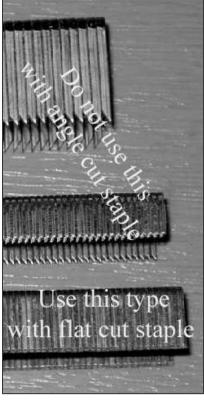
I USED STAPLES TO CLAMP THE PLYWOOD TO THE RIBS. THE STAPLES WERE LATER REMOVED AFTER THE GLUE HAD DRIED. THE PROCESS WORKED FINE EVEN THOUGHT IT MAY TAKE SLIGHTLY LONGER TO MAKE. THE KEY THING WITH STAPLES WAS TO FIND ONE TYPE THAT WAS FLAT IN THE BOTTOM PART. MOST COMMERCIAL HAD A ANGLE AT THE END WHERE IT FIRST GOES INTO THE MATERIAL. THAT WORKS GREAT
