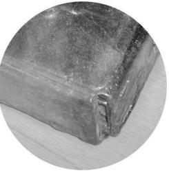
FOR ANYTHING BUT RIBS SINCE THE ANGLE CUT STAPLES WILL ROTATE SLIGHTLY WHEN MOVING DOWN IN THE MATERIAL. I FOUND HOBBY STAPLES WORKED OK BUT THEY HAD A TENDENCY TO BREAK OFF WHILE REMOVING THEM. THE BEST STAPLE THAT I FOUND WAS STANLEY 8MM (5/26). THE STAPLE-GUN WAS MODIFIED WITH A FEW PIECES OF 1MM PLYWOOD SO THAT THE STAPLE DID NOT GO DOWN ALL THE WAY FOR AN EASY REMOVAL.
